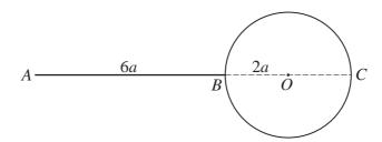
A rigid body consists of a thin uniform rod AB, of mass 4m and length 6a, joined at B to a point on the circumference of a uniform circular disc, with centre O, mass 8m and radius 2a. The point C on the circumference of the disc is such that BC is a diameter and ABC is a straight line (see diagram). The body rotates about a smooth fixed horizontal axis through C, perpendicular to the plane of the disc. The angle between CA and the downward vertical at time t is denoted by  $\theta$ .
